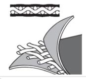
**Type C:** TRI-LAMINATE PVC sheet bonded to both sides of woven scrim
