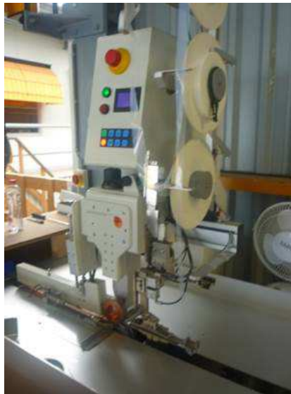
Ultrasonic head of a Jentschmann Weldsonic machine 2796-2-20
