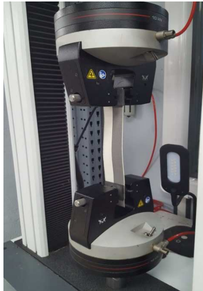
INSTRON "3000 series" dynamometer (Dickson Quality Laboratory)
