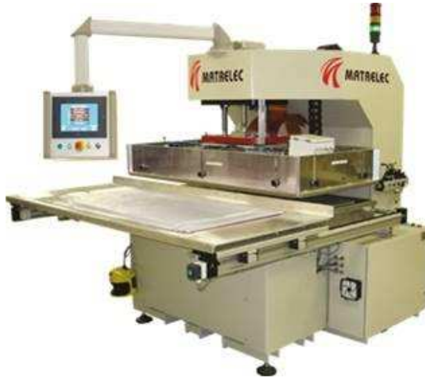
High-frequency 22 kW MATRELEC machine
