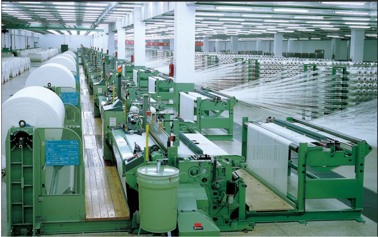
Figure Four (a) – A typical weaving mill, in this instance with yarn being inputted directly from bobbins, rather than a beam. The cards and shuttle (foreground machine) are located directly behind the drum in the centre of the picture.
