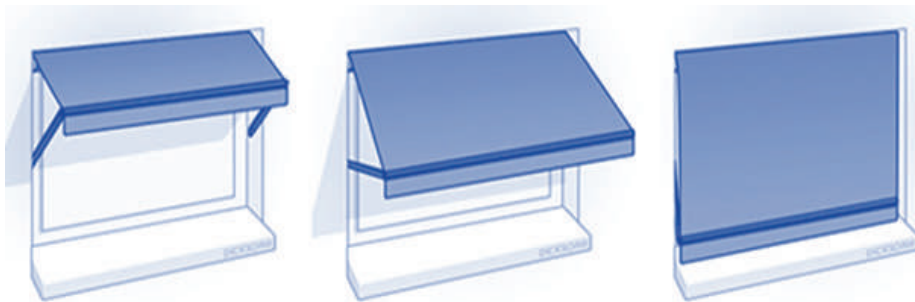
■ Figure Five - Typical Positioning of a Drop-Arm Awning, Determined by the Extent by Which the Fabric is Unrolled
