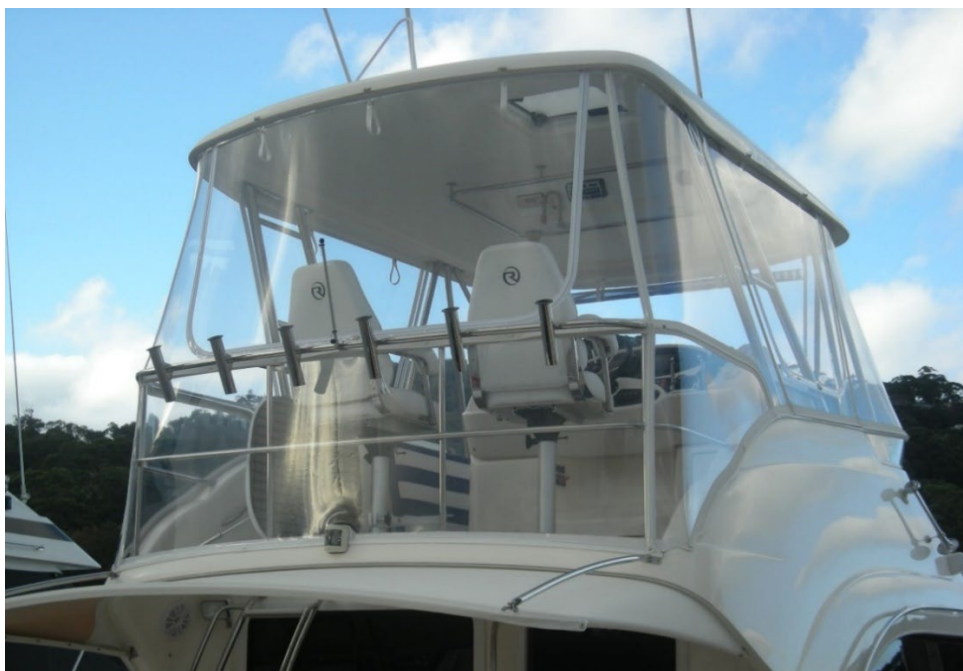
Figure Ten – An enclosure fabricated from Vybak Press Polished Clear PVC. This type of clear is preferred by high end boat owners because of its clarity.
