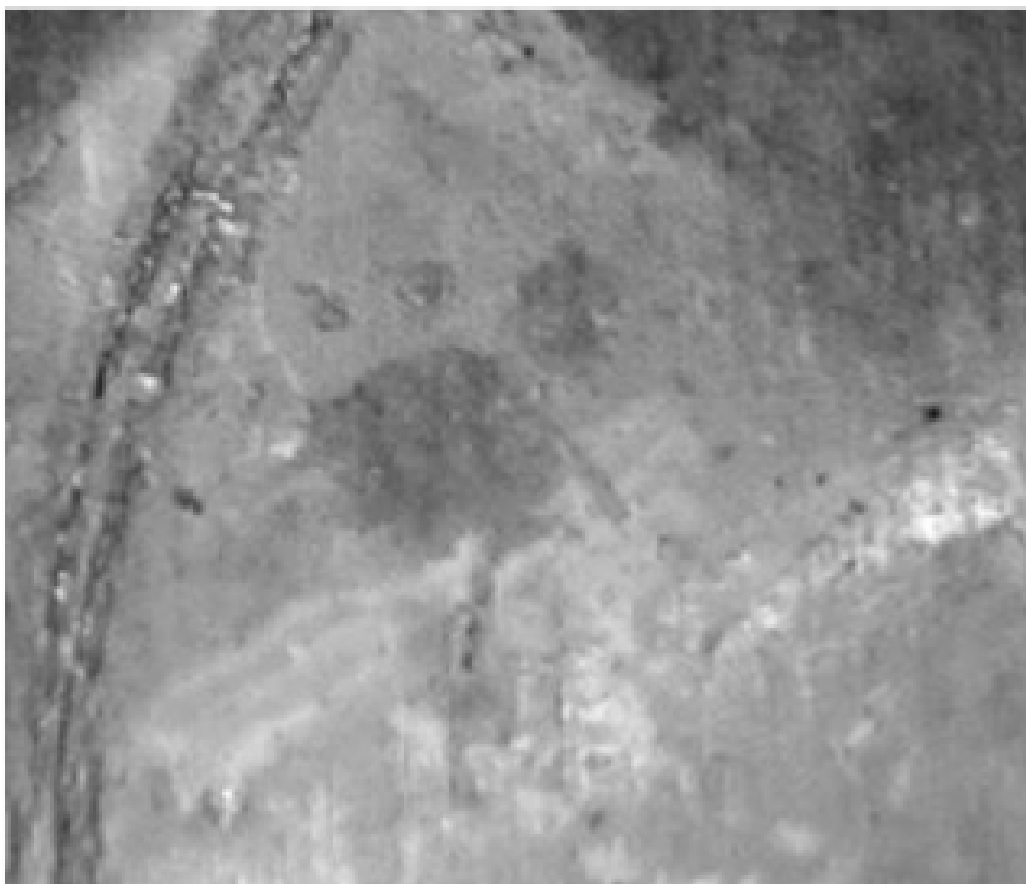
Figure Seventeen – Corrosion of Aluminium in contact with a stainless steel eyelet after only 48 hours immersion in a salt spray. The circular imprint of the eyelet (left) is clearly visible. (magnification x 10)
