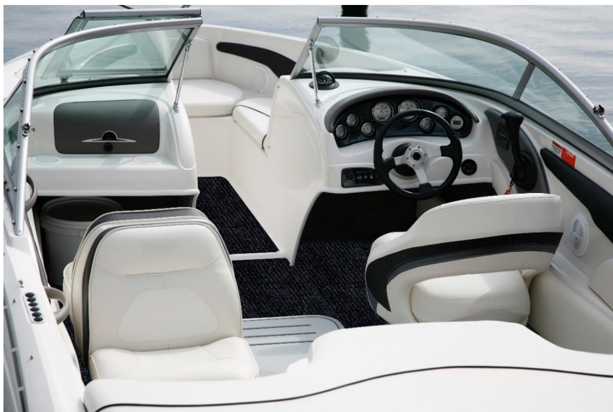
Figure Twelve – ‘Capri’ Expanded Upholstery Vinyl and ‘Four Seasons’ carpet used in a ski-boat. Both products display a high level of durability in the marine environment.
