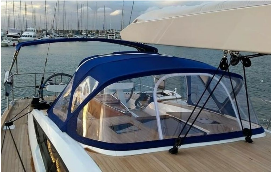
Figure Four – A ‘Dodger’, or ‘Spray Hood’, with Sunbrella fabric covering the frame, and flexible glazing (‘clears’) fabricated from Strataglass. Note the removable zippered windscreen, and the Bimini at the stern.
