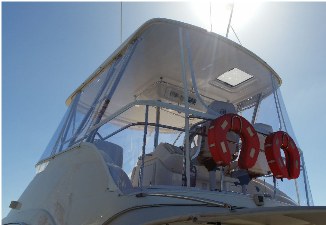
Figure Two – A ‘Bimini Enclosure’, or simply an ‘Enclosure’, as in this example it is attached to a fibreglass top. (Photo courtesy of Aussie Boat Covers)
