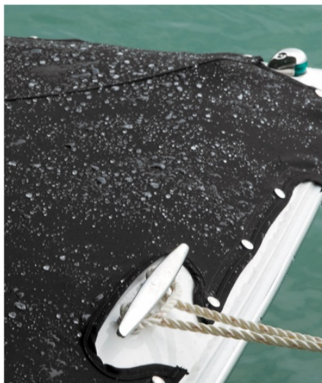
Figure Nine – The beading of water droplets on the surface of SunBrella Acrylic Fabric, caused by the polarising effect of the surface proofing, thus preventing leakage through the fabric.
