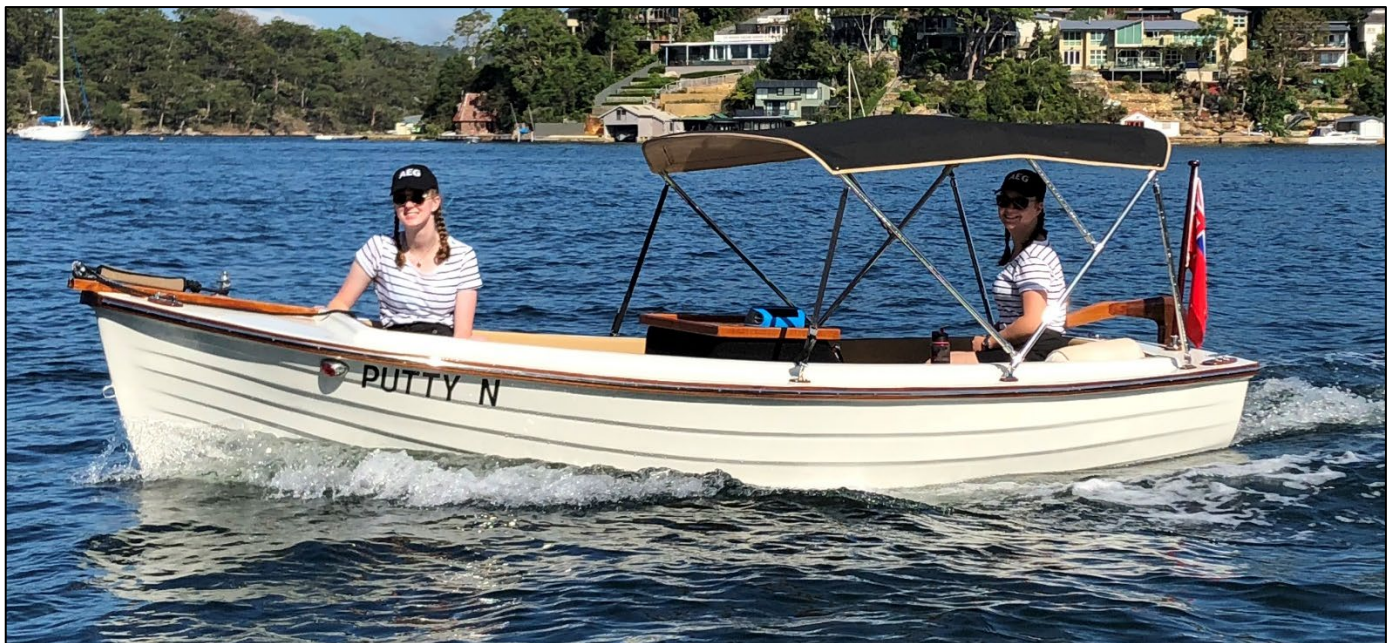
Figure One – A simple 'Bimini Top', fabricated from Sunbrella
