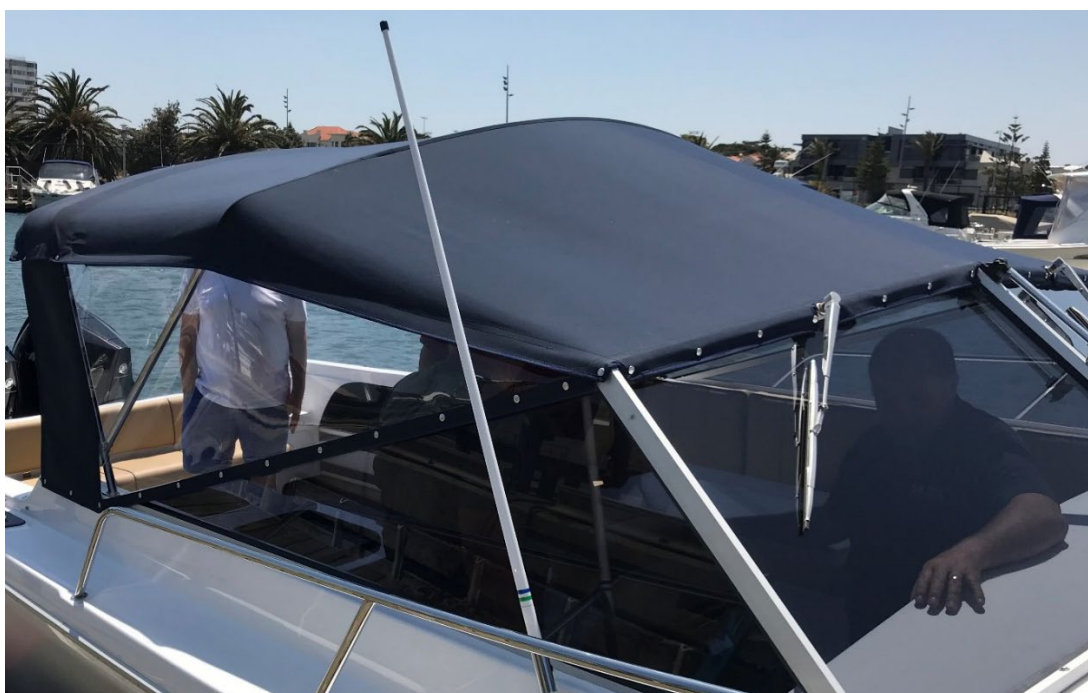
Figure Sixteen – A convertible top attached with ‘Durable’ fasteners. The use of the Perfix Q-snap at each corner of the windscreen greatly facilitates raising and lowering the top.
