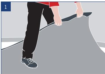
Wherever possible lay the carpet down the length of the room to minimise the number of cross joins. Avoid joins in doorways and high traffic areas. Measure the length of the room, and cut the first piece from the roll allowing extra for trimming at both ends. Ensure an allowance is made for doorways, alcoves and any irregularities of the walls. Starting at the corner furthest from the door, lay the first piece into position lapping the carpet up the walls at both ends for sufficient trimming.
