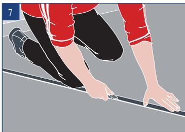
Position a straight edge along the middle of the overlap (join) and cut through both pieces of carpet with a sharp knife and remove the surplus. For ribbed carpets, the ribs should be aligned on both layers and the cut is made in the valley simultaneously. Fold back the seam edges and apply adhesive to the substrate where no adhesive is present. Re-lay the carpet and roll with a flooring roller to ensure overall contact with the adhesive.
