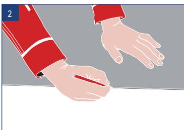
Run a pencil along the inner edge of the carpet making a guide line on the floor for the application of adhesive.
