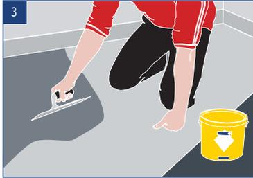
Fold the sheet half way back taking care not to disturb the positioning of the flooring. Apply the recommended adhesive onto the subfloor, from the wall to within 10cm of the guide line. Replace the carpet carefully and accurately back into position and roll with a flooring roller to ensure adhesive transfer to the back of the carpet. Repeat for the other half of the sheet.
