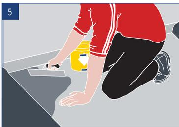
Fold the sheet half way back taking care not to disturb the positioning of the flooring. Apply the recommended adhesive onto the subfloor using the application techniques previously described, from 10cm inside the first guide line to 10cm inside the next. Replace the carpet carefully and accurately back into position and roll with a flooring roller. Repeat for the other end of the sheet. Successive lengths may be installed in this way.
