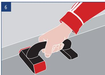
Using an Araseur or a sharp knife and trim the carpet to fit against the perimeter walls.
